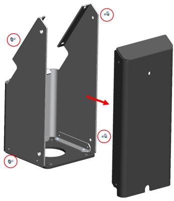
Remove and save (4) screws from stand with provided hex wrench, pull off rear cover.
