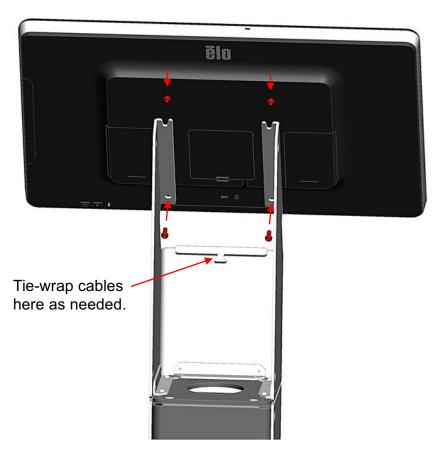
Assemble (2) screws from bag "I" to the top two VESA mount holes on the display. Assemble the display to top slotted holes on stand. Add additional (2) screws from bag "I" to bottom VESA mount holes to secure the display.
