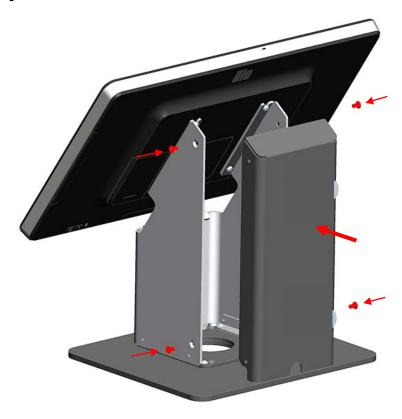
Route cables through bottom of stand. Attach back cover using screws saved from step 1.
