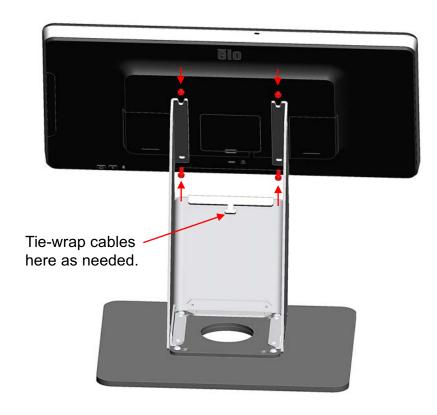
Assemble (2) screws from bag "I" to the top two VESA mount holes on the display. Assemble the display to top slotted holes on stand. Add additional (2) screws from bag "I" to bottom VESA mount holes to secure the display.
