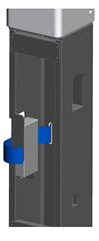
Add power brick into tower using provided strap. Route additional cables through base, tower, head as needed. 9
