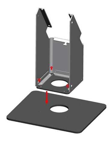
Attach head to counter top plate using (4) screws from bag "I".
