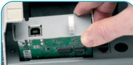
Easily interchangeable interfaces - USB, Ethernet, Serial, Parallel and WebPRNT
