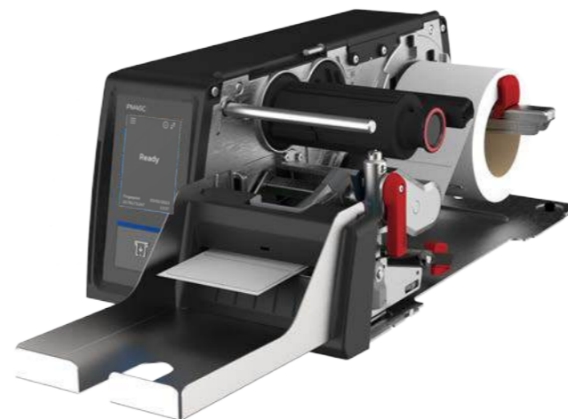
Horizontal Tray installed
