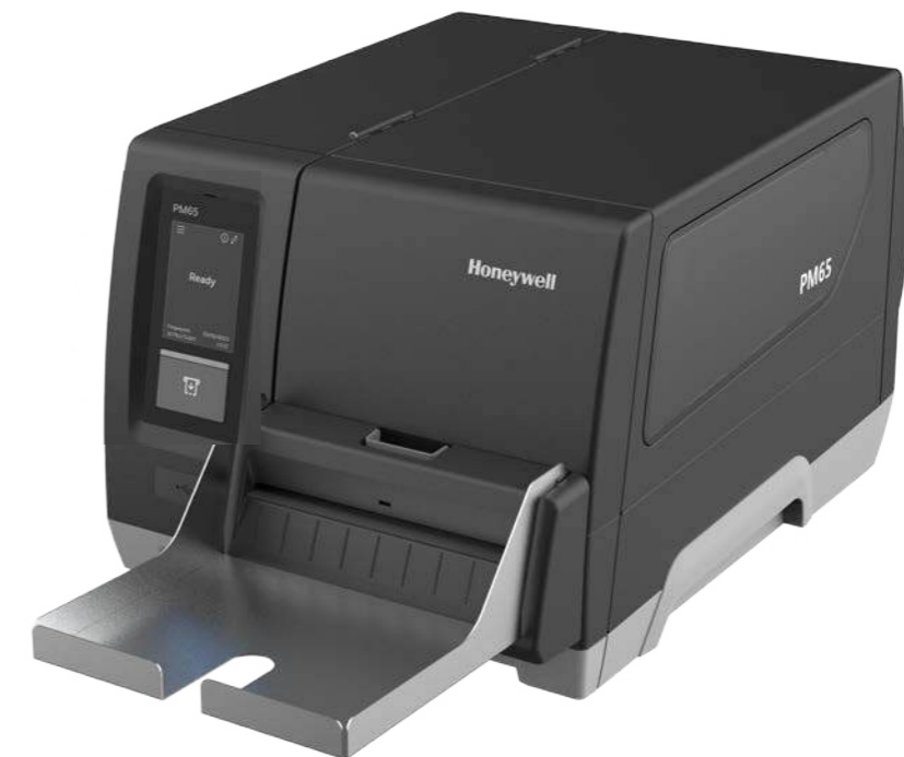
PM65 with Cutter (Side Door)
