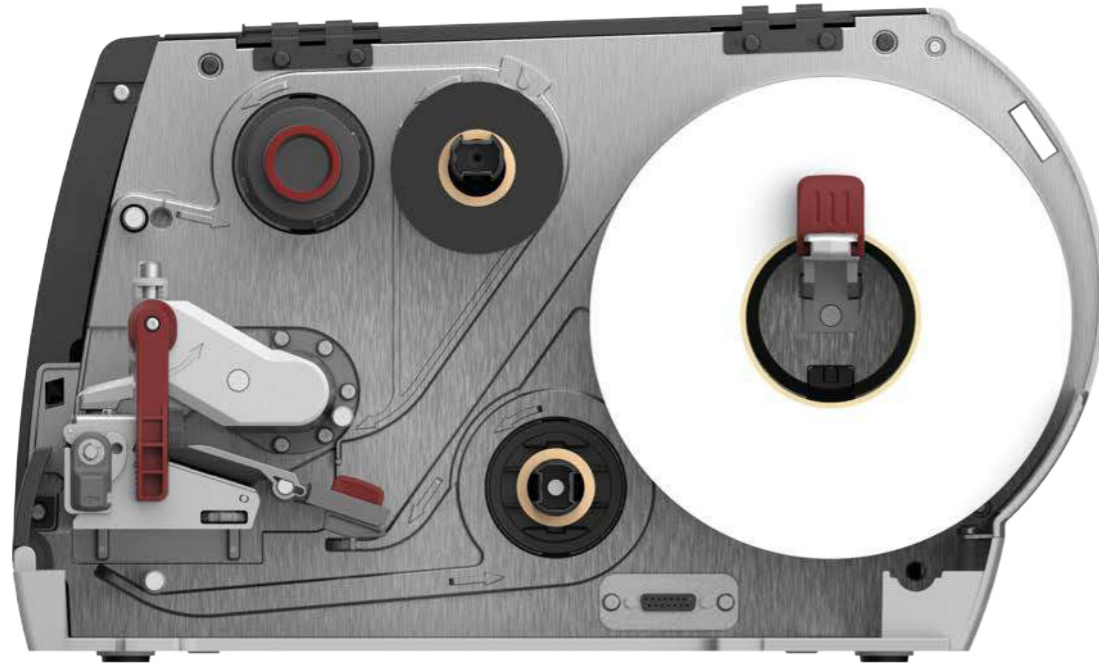
Fixed Media Hanger + Label Roll Core 76 mm (3.0 in) ID Shown with Label Roll 213 mm (8.38 in) OD Typical length of material with typical thickness of labels ~ 195 m
